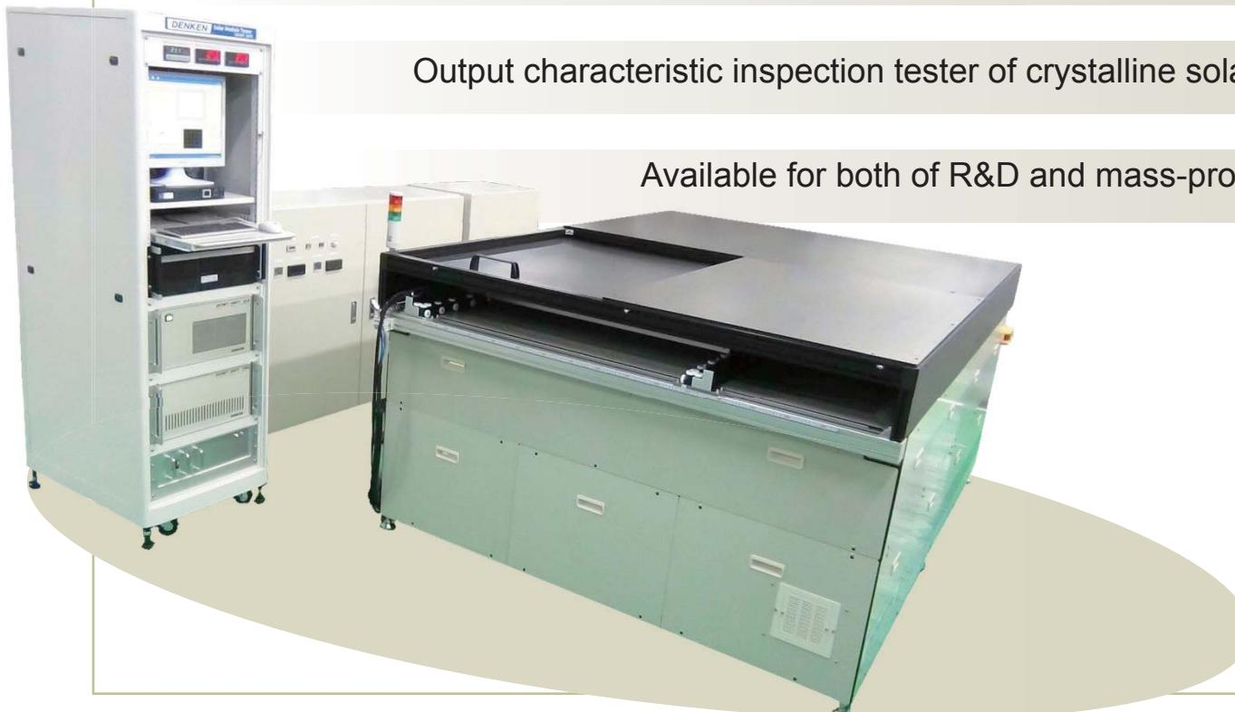
Output characteristic inspection tester of crystalline solar cells
